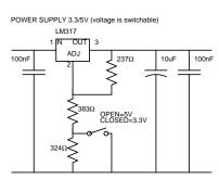
Figure 4: i2c powerizer power supply circuit options
