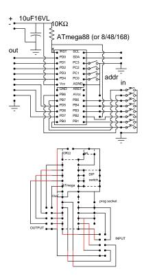
Figure 3: i2c Powerizer schematics
