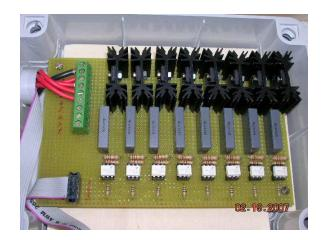
Figure 2: A picture of an eight channel Digital Powerizer
