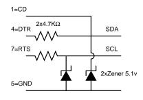
Figure 5: i2c to PC serial port interface
