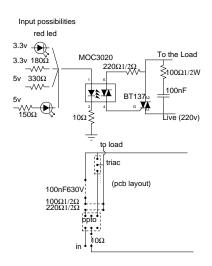
Figure 1: Digital Powerizer schematics
