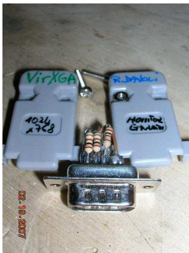
Figure 3: VirXGA prototype (inside view)
