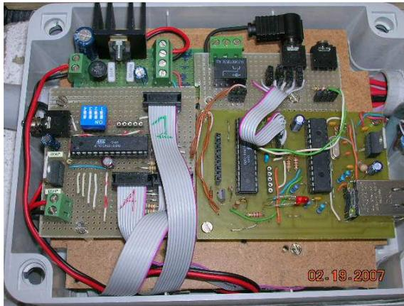
Figure 6: A picture of an i2c-Powerizer (lower left corner) in a box with an Ethernet controller
