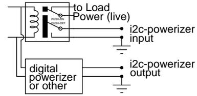
Figure 7: i2c powerizer connected to a push-on push-off relay (addr i= 8)
