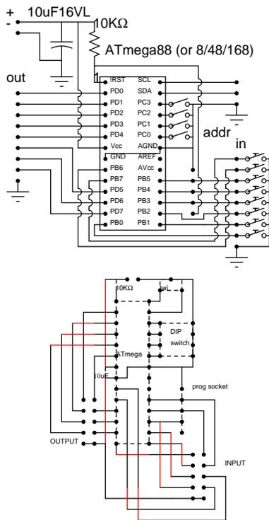
Figure 3: i2c Powerizer schematics
