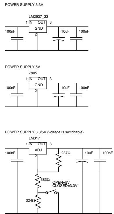
Figure 4: i2c powerizer power supply circuit options
