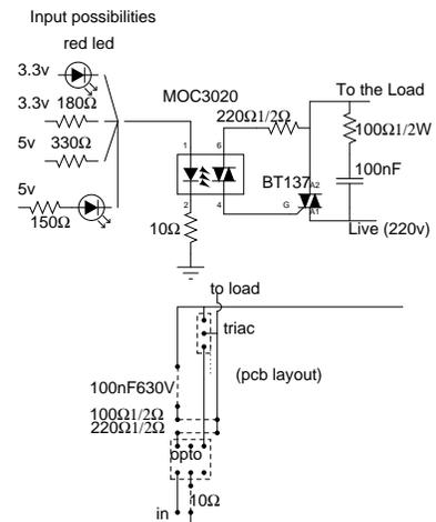
Figure 1: Digital Powerizer schematics
