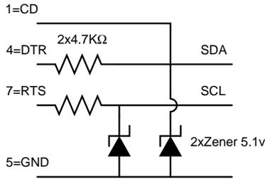
Figure 5: i2c to PC serial port interface
